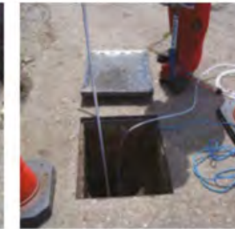
3. Remove lance and disconnect pump
